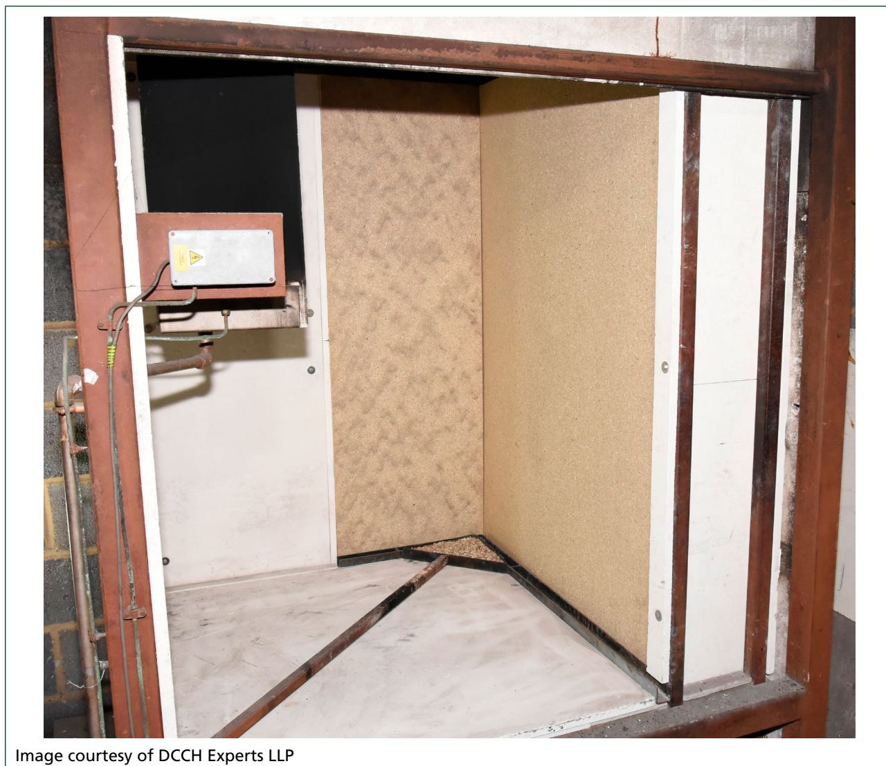
Figure A.5 – BS EN 13823 test apparatus with blank specimen in position for test
