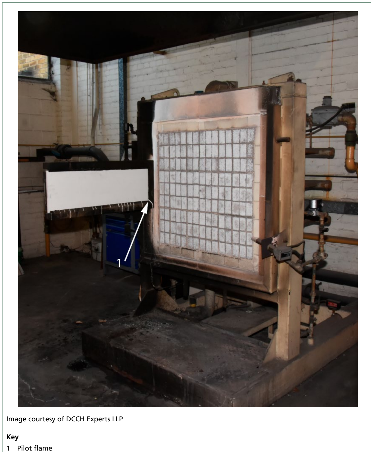
Figure A.1 – BS 476-7 test apparatus with specimen holder in position for test and containing a blank specimen
