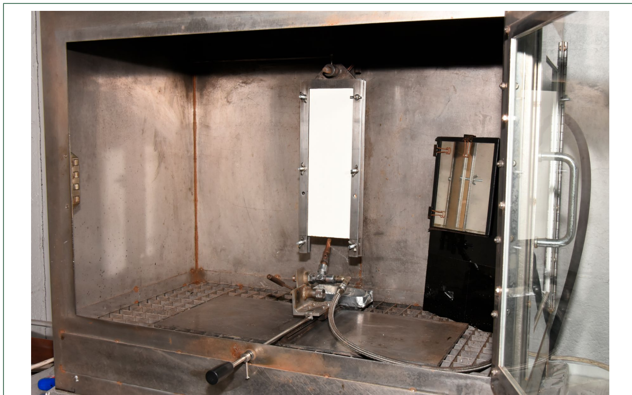
Figure A.4 – BS EN ISO 11925-2 test apparatus with blank specimen in position for test
