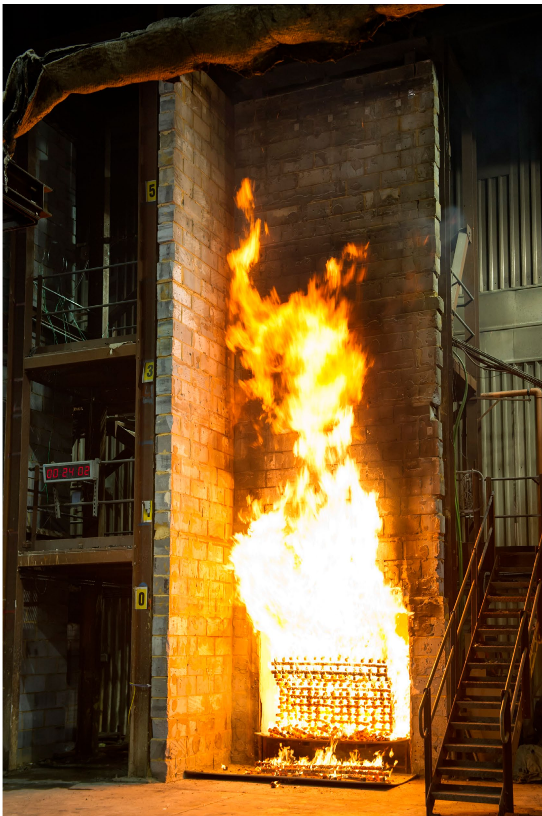
Figure A.10 – BS 8414-1 rig with a timber crib fully alight but no specimen installed, indicating severity of test when there is no contribution from a test specimen
